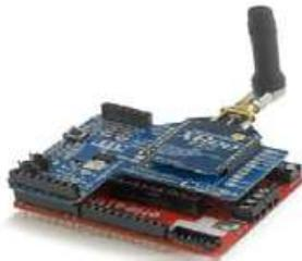
Figure 7: Arduino using Zigbee protocol [9]
